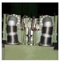
UM type expansion joints installed on an engine.
