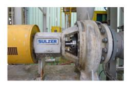
An EagleBurgmann **MA291/60** type single cartridge seal is installed in a Sulzer APP pump at an Indonesian paper mill. The medium to be sealed is pulp with a solids content of 5.5 %. Operating conditions: p = 4 bar (58 PSI), t = 60 °C (140 °F),  $n = 1,430 min^{-1}$ .
