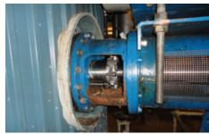
After retrofitting at Stora Enso in Sweden, two fully split EagleBurgmann **Splitex** type mechanical seals operate successfully in a mixer with bottom entry and a chest agitator with side entry. Here, pulp having a solids content of over 11 % is sealed. Operating conditions: p = 10.3 bar (149 PSI), t = 180 °C (356 °F), n = 15 min<sup>-1</sup>.
