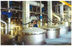
At UPM Kymmene Shotton in England, nine Voith pressure screens in waste paper treatment are being used successfully with EagleBurgmann  $\mathbf{HR-D}$  type double cartridge seals. Medium to be sealed: Pulp fibers 1.5 ... 4 % abs. dry and water, p=8 bar (116 PSI), t=max. 40 °C (104 °F).
