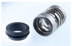
**HA211** type mechanical seals operate in the fiberization process of the mechanical pulp production at Nippon Paper in Japan to provide secure sealing of white water. Operating conditions: p=1 bar (15 PSI), t=30 °C (86 °F), n=1,450 min<sup>-1</sup>.
