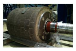
UPM Plattling/Germany uses Metso pressure grinders to fiberize wood. EagleBurgmann  $\begin{tabular}{l} HSSHR8-D4/470-E1 type mechanical seals are used to seal off both sides of the high-consistency groundwood pulp at the grindstone shaft. Operating conditions: p = 3 bar (44 PSI), t = 150 °C (302 °F), n = 350 min <math>^{-1}$ .
