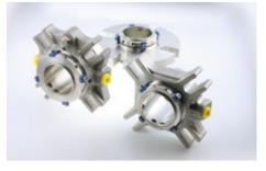
A successful seal type for the entire plant: Over 250 standardized EagleBurgmann Cartex cartridge seals are installed in pulp pumps and in the pumps of the chemical sector at the Swedish Iggesund Holmen paper and pulp mill. Operating conditions: p = 12 ...25 bar (174 ... 363 PSI), t = -40 °C ... +220 °C  $(-40 \text{ °F } \dots +428 \text{ °F}), n = 1,660 \text{ min}^{-1}.$
