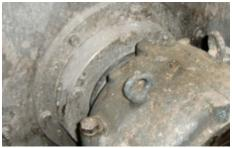
A horizontally arranged machine shaft is sealed by an Espey **E-WDKS205** type carbon floating ring seal at Norske Skog Saugbrugs in Norway. Operating conditions:  $t = 40 \, ^{\circ}\text{C} \dots 50 \, ^{\circ}\text{C} (104 \, ^{\circ}\text{F} \dots 122 \, ^{\circ}\text{F}), \, n = 11 \dots 15 \, \text{min}^{-1}.$
