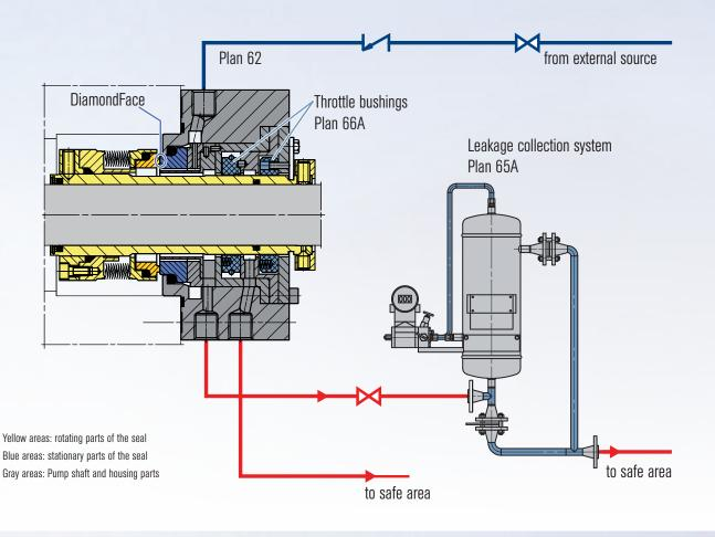
Cross section of the mechanical seal MFLWTI with Plan 66A, supply according to API Plan 62 (steam quench from external source), leakage collection and alarm system LSA6 according to Plan 65A. The sliding faces of the seal are coated with DiamondFace.
